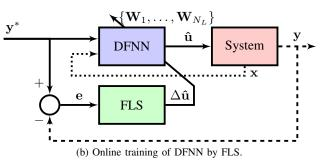
Fig. 3. Block diagrams of the two control paradigms: offline pre-training and online training (solid lines represent calculated quantities, dashed lines represent measured quantities, dotted lines represent estimated quantities).
