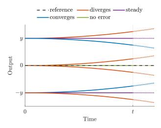
Fig. 4. Possible evolution of the controlled dynamical system. The system can diverge (red curves), converge (blue curves), it can have a steady error (purple lines), or the error can be zero (green line). In the proposed approach, FLC observes the time evolution of the output from the system controlled by DFNN and, depending on the situation, corrects the action of DFNN.
