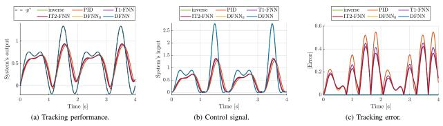
Fig. 6. Simulation results for different controllers on the nominal system in (28). It is possible to observe that both DFNN<sub>0</sub> and DFNN with online learning are able to track precisely the desired trajectory of the nominal system. In addition, DFNN<sub>0</sub> approximates accurately the exact inverse of the system in (6).
