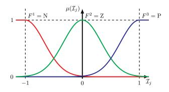
Fig. 2. "Negative" (N), "zero" (Z) and "positive" (P) FSs represented by three Gaussian MFs.
