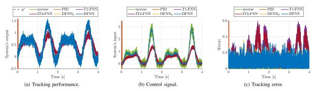
Fig. 9. Simulation results for different controllers on the nominal system with noisy measurements in (31). It is possible to observe that PID controller is not able to deal with this level of noise. While all T1-FNN, IT2-FNN DFNN<sub>0</sub> and DFNN are able to control the system.
