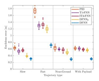
Fig. 15. Box-plot of the tracking performances of five controllers in four scenarios. For each controllers-scenarios case, the experiments are repeated five times under quasi-same conditions. It is possible to observe that DFNN-based controller with online learning has the lowest maximum absolute error, even for the cases unseen during the pre-training.
