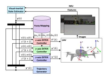
Fig. 10. Illustration of the proposed online learning-based control scheme. During the online learning phase, DFNN controls the UAV and, by using the expert knowledge encoded into the fuzzy mapping, improves further the performance in real-time.
