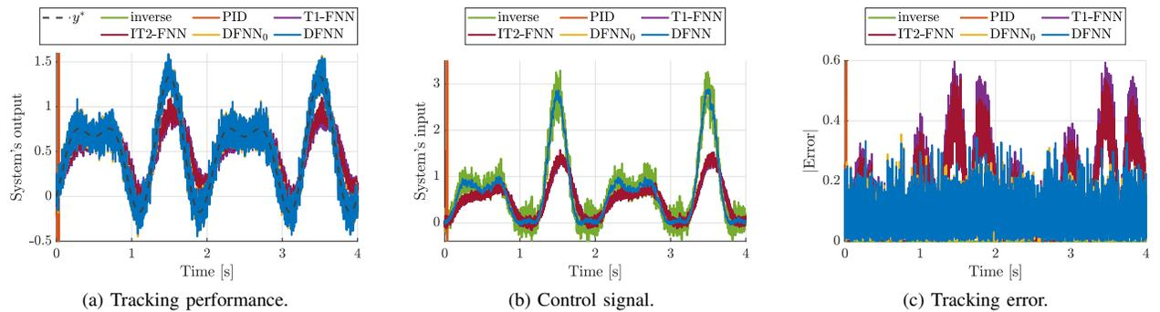
Fig. 9. Simulation results for different controllers on the nominal system with noisy measurements in (31). It is possible to observe that PID controller is not able to deal with this level of noise. While all T1-FNN, IT2-FNN, DFNN<sub>0</sub> and DFNN are able to control the system.
