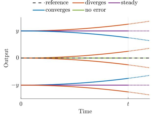
Fig. 4. Possible evolution of the controlled dynamical system. The system can diverge (red curves), converge (blue curves), it can have a steady error (purple lines), or the error can be zero (green line). In the proposed approach, FLC observes the time evolution of the output from the system controlled by DFNN and, depending on the situation, corrects the action of DFNN.
