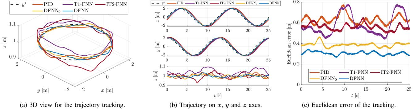
Fig. 11. Experimental results for different controllers on the slow circular trajectory at velocity of 1m/s.
