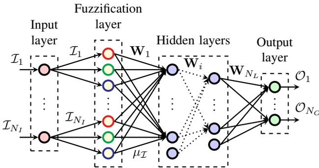
Fig. 1. Structure of DFNN organized in input layer with  $N_I$  neurons, Gaussian fuzzification layer with  $N_F$  neurons,  $N_L$  fully-connected hidden layers with  $(N_H + 1)$  neurons in each layer and output layer with  $N_O$  neurons.
