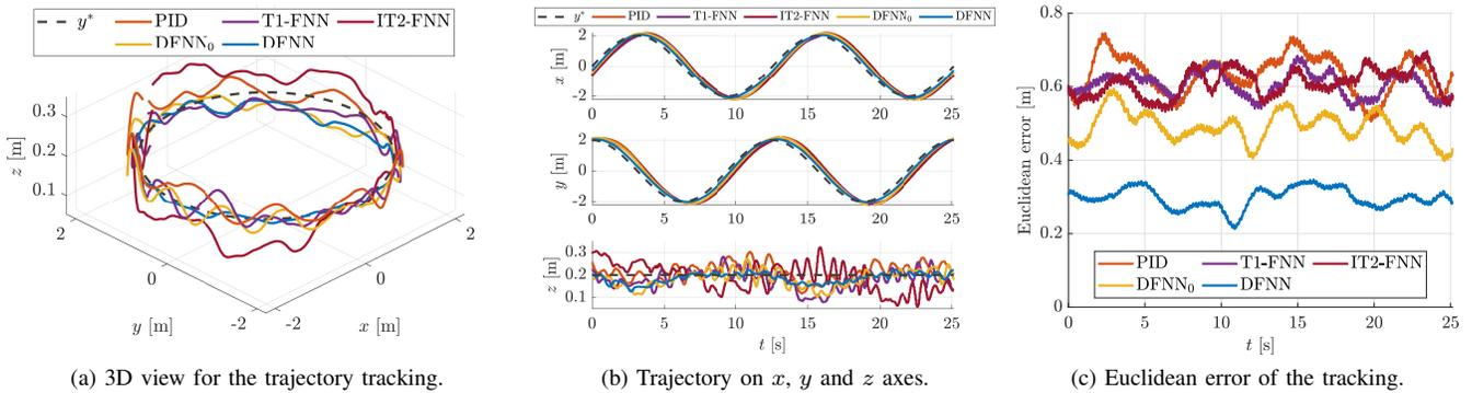
Fig. 13. Experimental results for different controllers on the near-ground circular trajectory at height of 0.2m.
