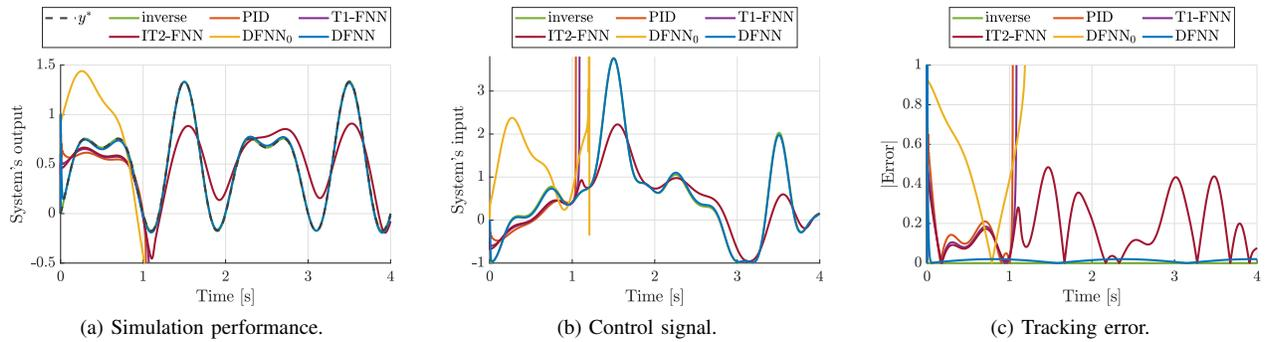
Fig. 8. Simulation results for different controllers on the nominal system with external time-varying disturbance in (30). All PID, T1-FNN and DFNN<sub>0</sub> become unstable with time-varying disturbance. While DFNN with online learning is able to learn the new conditions and obtain good performances.
