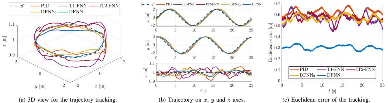
Fig. 14. Experimental results for different controllers on the circular trajectory with payload of 209g.
