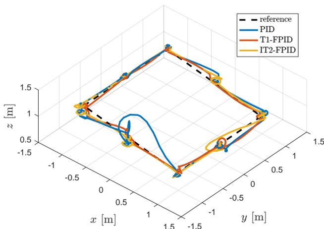
Fig. 11. Trajectory tracking in 3D space in presence of wind.
