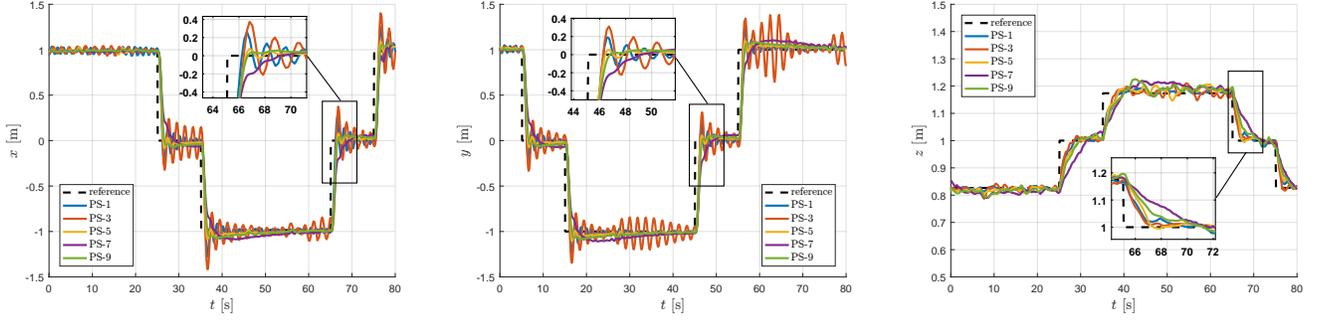
Fig. 8. Trajectory tracking for  $x$ ,  $y$  and  $z$  axes of SI-IT2-FPID position controllers with different values of  $\alpha_p$  and  $\alpha_d$  in absence of wind.
