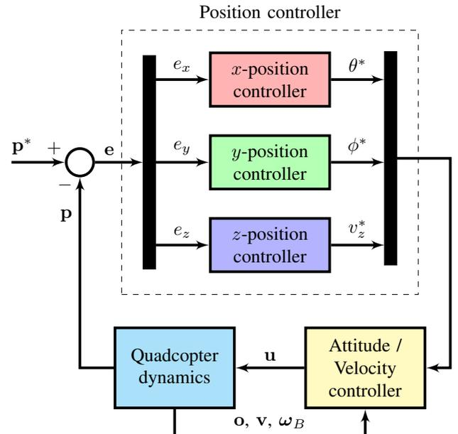
Fig. 2. Block diagram of the control system for the quadcopter UAV.
