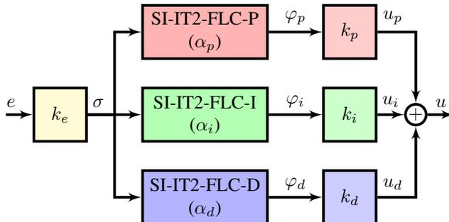
Fig. 3. Structure of the SI-IT2-FPID position controller.
