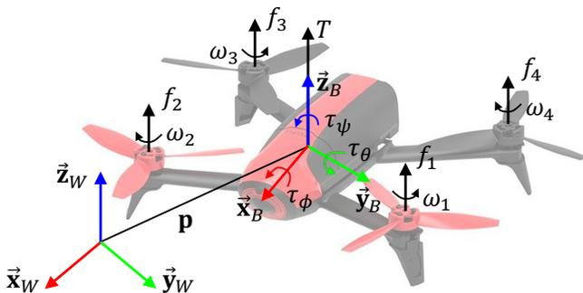
Fig. 1. Parrot Bebop 2 quadcopter UAV with its reference frames.
