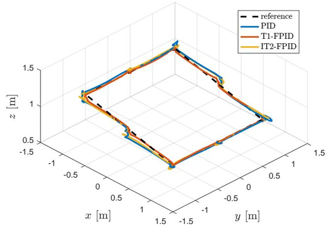
Fig. 9. Trajectory tracking in 3D space in absence of wind.
