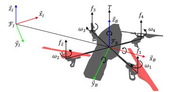
Fig. 1: Quadrotor UAV model with reference frames.
