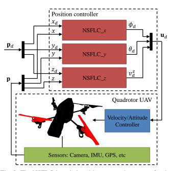
Fig. 2: The NSFLC-based closed-loop control structure for the navigation of the quadrotor UAV.
