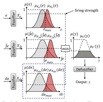
Fig. 3: Example of the calculation from inputs  $(X_*)$ , antecedents  $(A_*)$  and consequent (C) fuzzy sets to output (Y) of a Sta-NSFLC.
