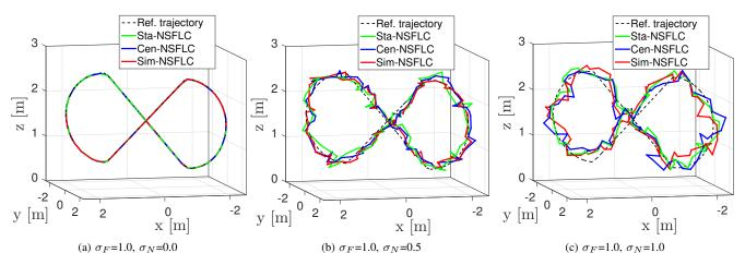
Fig. 6: Example of three UAV flights with the same input fuzzification ( $\sigma_F$ =1.0) under three different levels of noise.
