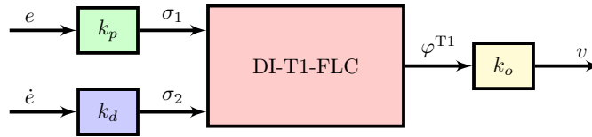
Figure 2: Structure of DI-T1-PPD controller.
